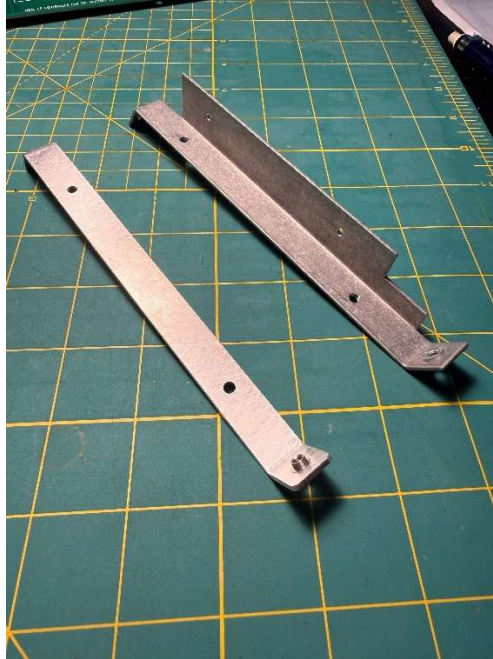
Figure 2 - Flat and "L" style heat sink brackets.
