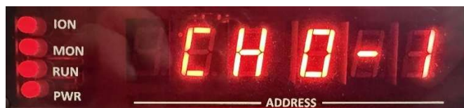
Figure 12 - Front Panel Display After Initiating Boot.
