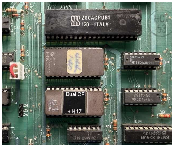
Figure 10 - Modified XCON-8 ROM with CF Boot Installed in U19.
