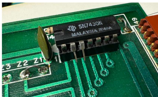
Figure 8 - Modifying IC207 on 8080 CPU board.
