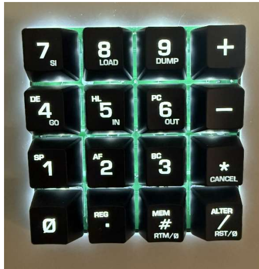
Figure 11 - H8 Front Panel Monitor Keypad.
