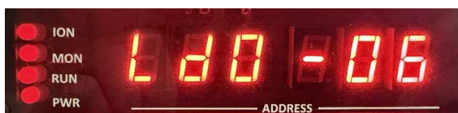
Figure 13- Front Panel Prompt to Select Boot Image.
