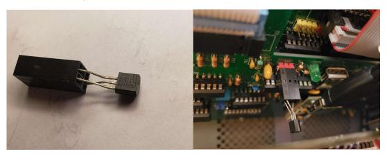
The TL7757 keeps the RESET line low (active) until power has stabilized:
