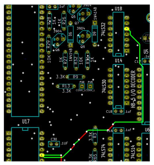
5.0 On side 2, solder a wire from U18 pin 6 to U11 pin 11 as shown.
