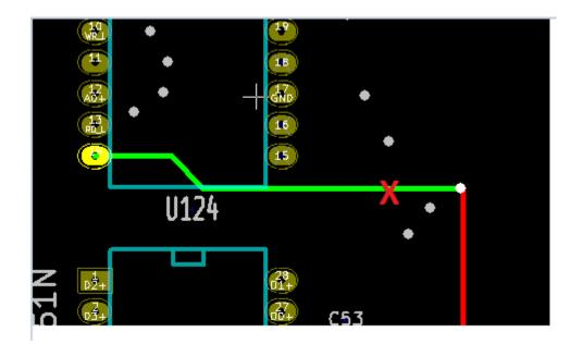
2.0 On side 2, solder a wire from U124 pin 14 to U112 pin 13 as shown.
