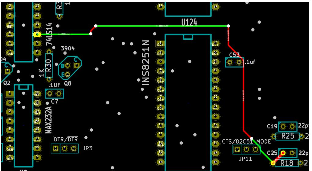
6.0 On side 2, solder a wire from U11 pin 10 to R18 pin closest to JP11 as shown.
