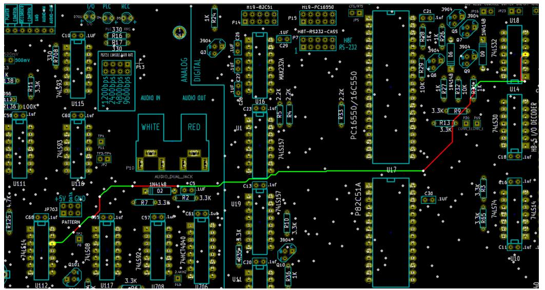
3.0 On side 2, solder a wire from U112 pin 12 to U18 pin 4 as shown.
