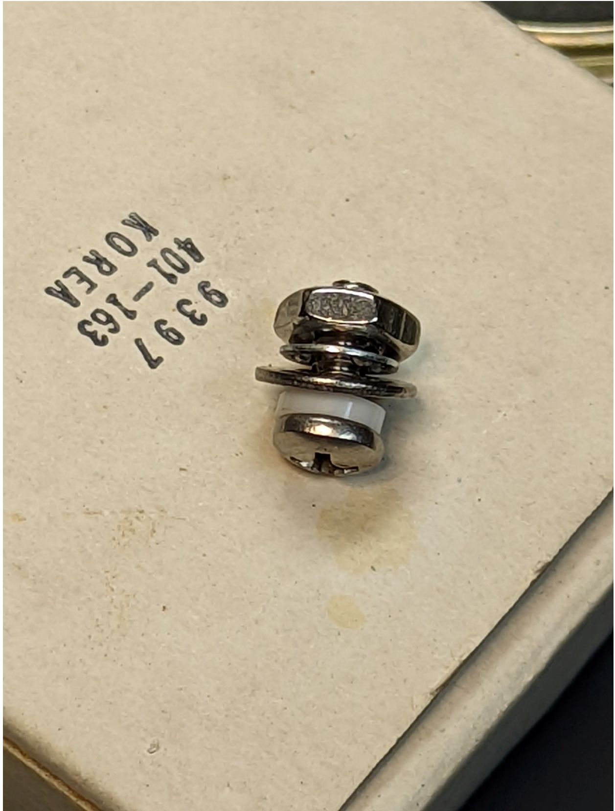
The 1/16" spacer and #6 flat washer duplicate the dimensions of the shoulder nuts that Heath used.
