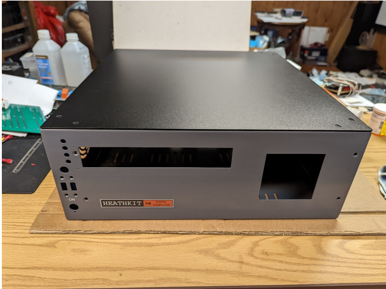
Countersinking of top fasteners gives a top with no protrusions (Glenn's good idea).
