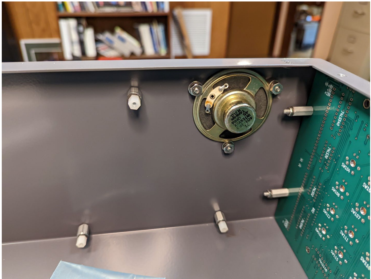
The speaker mounts to the case using built-up shoulder washers shown on the next page.
