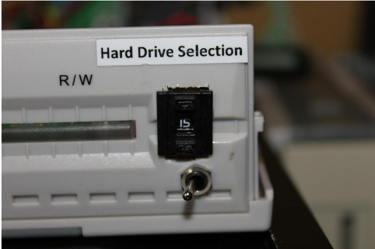
Hex switch – Position from 0 to 15 (with 4GB CF card). Switch below is to enable from Drive 16 to 32 with 8GB CF cards, and not required when using 2GB or 4GB CF cards.
