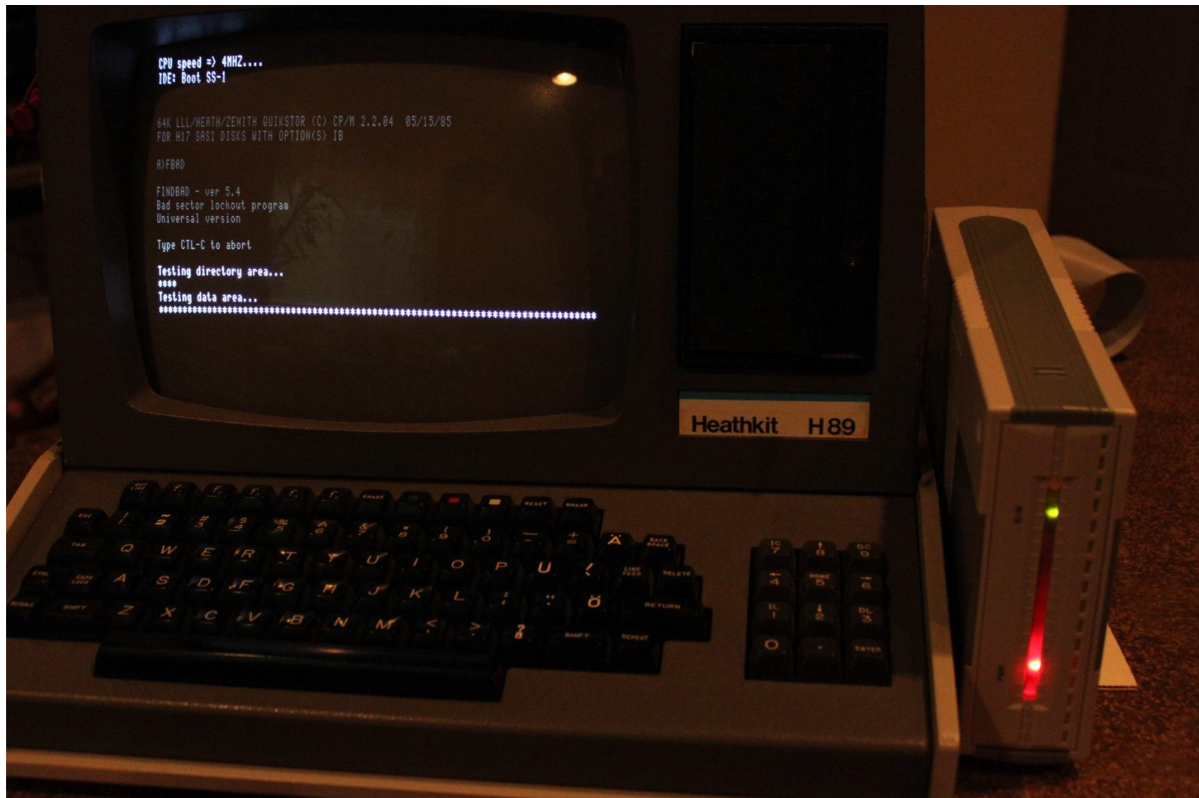
H89 booting CP/M from the Z67-IDE board
