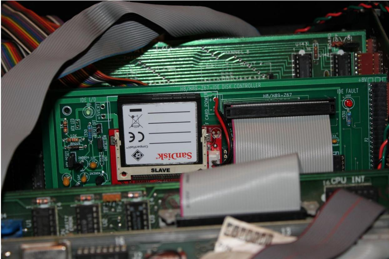
Figure 22: Z67-IDE board inside the H8 Chassis – Attached to the WH-8-37 Controller
