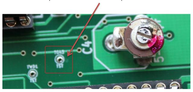
2. Adjust the RPW (R12) potentiometer for 1us as shown below.
