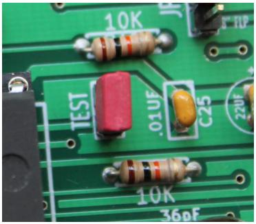
6. Connect scope probe to the "TWD1" test pin as shown below
