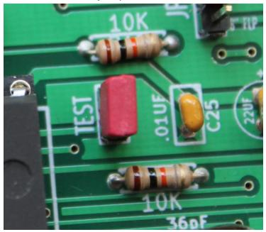
5. Using the DVM observed the voltage on the "10K" test point (WPW1) and ground as shown below. Adjust WPW potentiometer (R13) for the desired voltage of **1.340** volts
