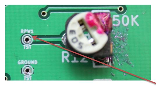
3. Adjust RPW potentiometer (R12) for the desired voltage value of **1.516** volts
