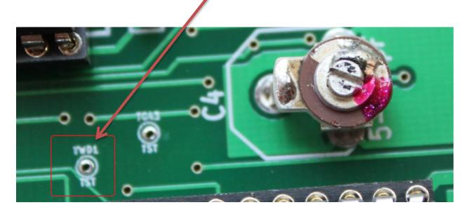
7. Adjust WPW potentiometer (R13) for the desired pulse width of 200ns as shown below.
