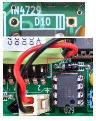
✓ Insert external battery. Observed polarity + (red cable) and – (black cable).
