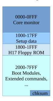
The core monitor contains the code to enter and execute commands and perform basic system initialization and management. It also contains the code to search the boot modules. There are also some well-defined entry points into the core monitor, which may be used by boot modules or even standalone programs.
