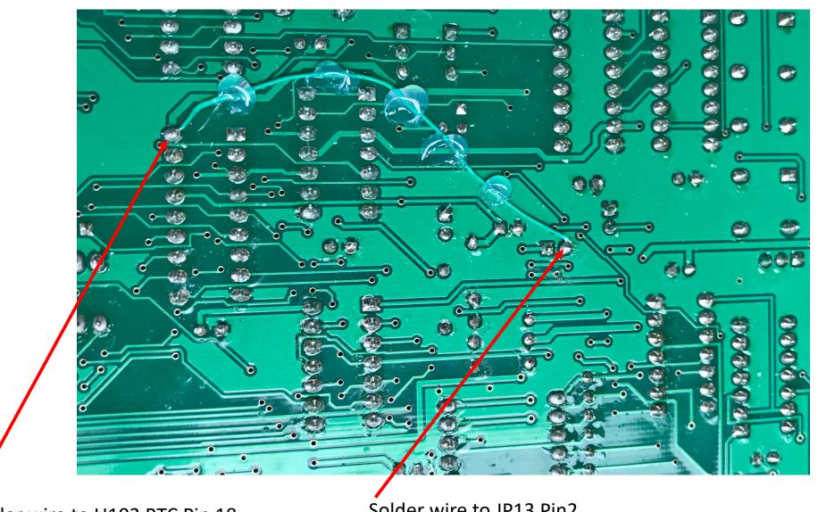
Solder wire to U103 RTC Pin 18
