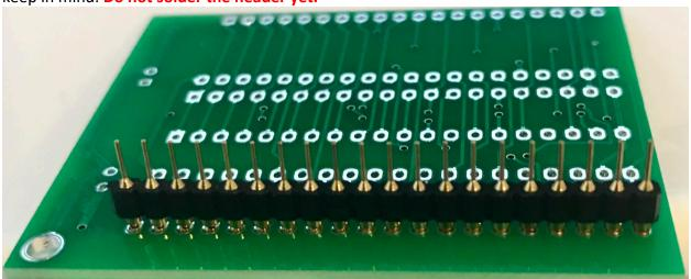
4. Locate on the Z80 board U114 DUART 40 pin machined socket. Insert the 20-pin header with the round pins facing out as shown.
