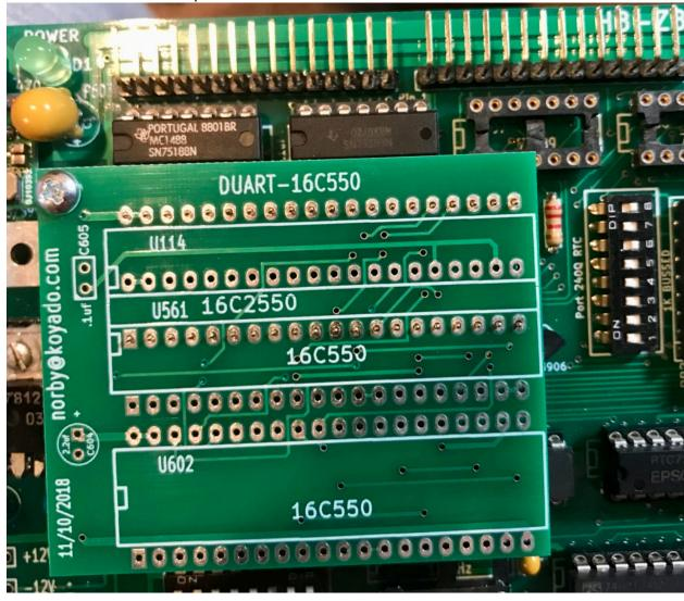
7. While pushing down on the middle of U114, solder the 2x20 male pin headers from the top of the board as shown below.
