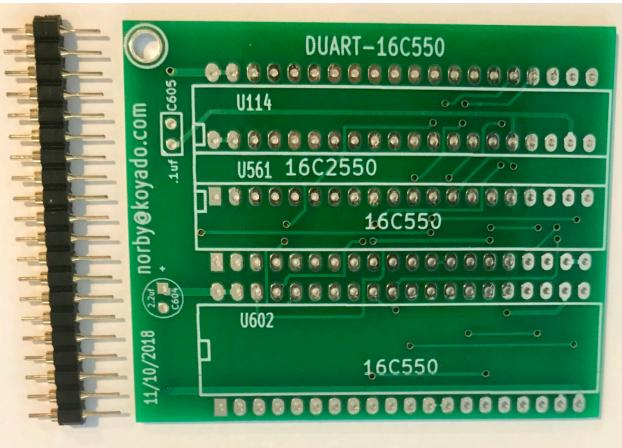
3. The round pins will be soldered to the DUAL board as shown below. This is important to keep in mind. Do not solder the header yet.
