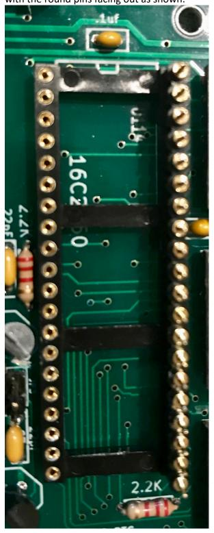
5. Insert the remainder 20-pin header as shown below.
