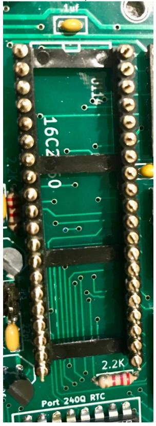
6. Placed DUART board on top of U114 as shown below.
