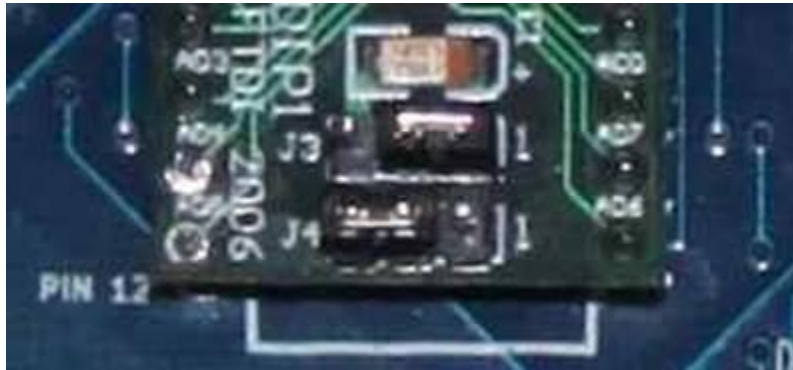
Two three way jumper pin headers are provided to allow for simple configuration of the I/O on data and control bus pins of the VDIP1. This is done by a combination of pulling up or pulling down the VNC1L ACBUS5 (pin 46) and ACBUS6 (pin 47). The relevant portion of the VDIP1 module schematic is shown in Figure 3.2
