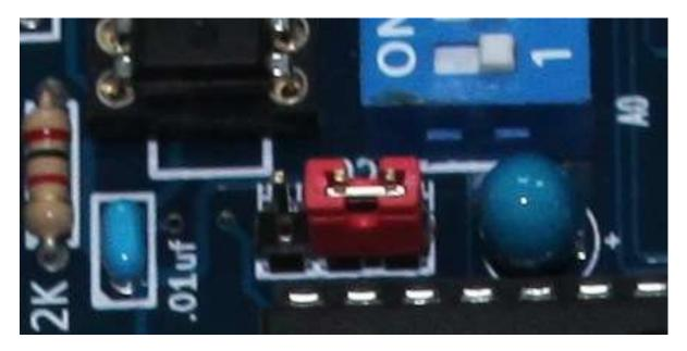
3. Set JP5 to "24.576 MHZ" position to enable secondary oscillator. Usually this secondary oscillator is a 10MHz part when using a 10MHz Z80 CPU. Beyond 10 MHZ a Z84C0020 is required.
