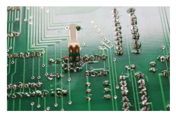
Solder a two pin right angle header on side two of the Z80 board as shown above.
