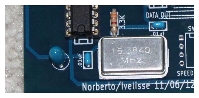
( ) Using the soldering iron on a "14 Pin Machine Tooled Low Profile Soldertail" socket (JAMECO P/N: 37197), remove pins 2, 3, 5, 6, 9, 10, 12, 13. Solder part into OSC # 2 position. This socket allows using half or full cans oscillators.
