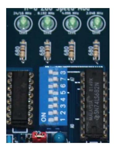
3. Configure the 4-position speed switch as follows for max speed selection; Switch 1, 2, and 3 = OFF and switch 4 = ON as shown below.
