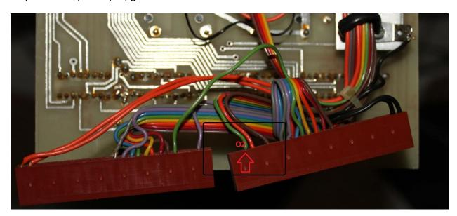
Step 4: Take out O2 green cable from pin 22 and insert it into pin 24 as shown below
