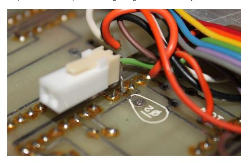
Step 6: Solder two pin header to ground. Also connect O2 green cable to ground as shown
