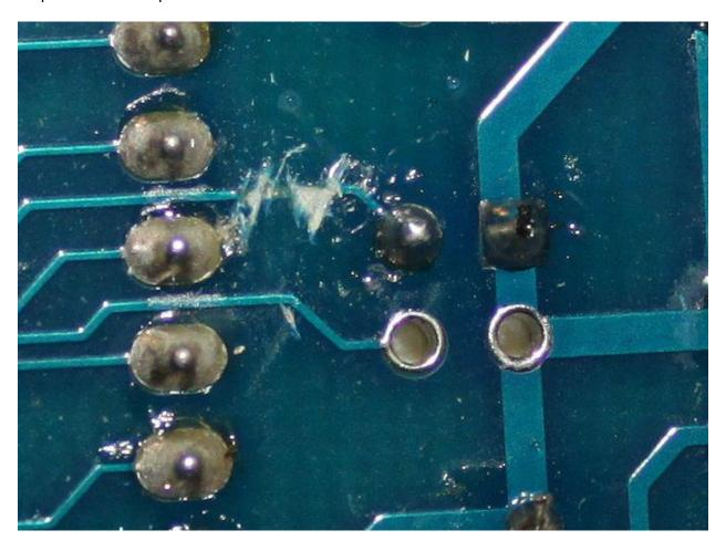
Step 10: On the H8-Speed board solder wire-wrap cable from U8 pin 6 to the two pin header as shown
