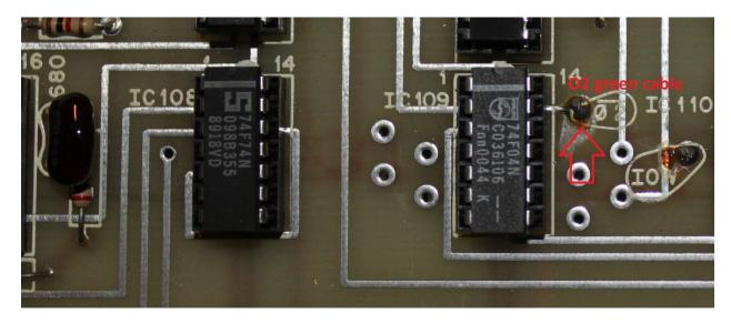
Step 6: Solder a two pin header right angle on side two to pin 13 of IC109 as shown
