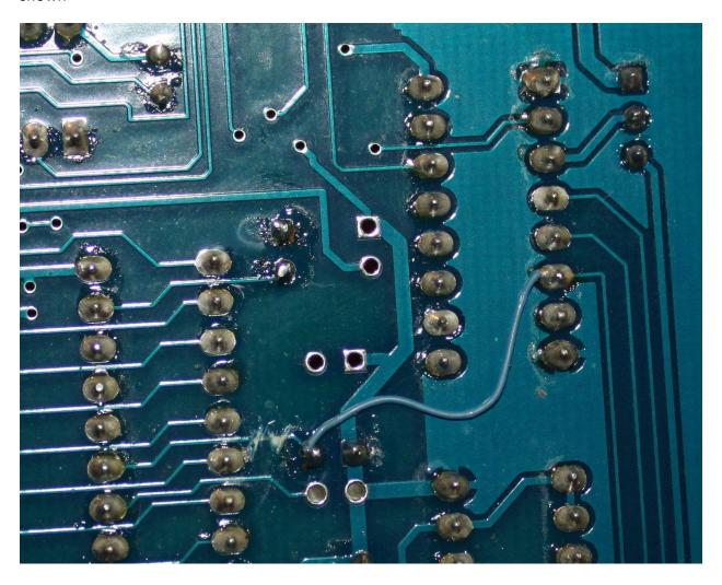
Step 11: Solder a two pin header in D3+R position on side 1 and connect coaxial cable
