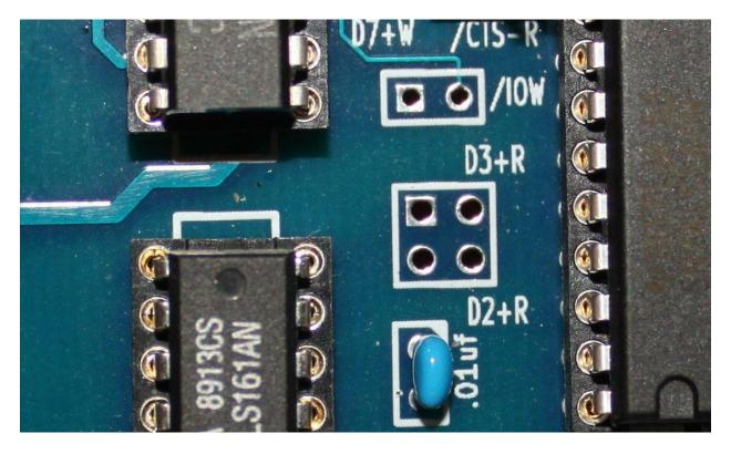
Step 9: On the H8-Speed board cut trace as shown on D3+R side
