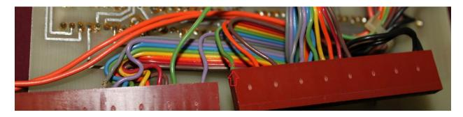
Step 5: Remove the other end of the green cable from the PCB board.
