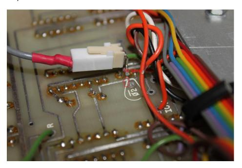
Step 8: On the H8-Speed board located 4-pin header D3+R/D2+R
