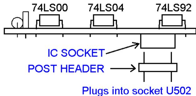
2. Examine the board to get the proper orientation. The front side of the board should have the letters "Rev: 1.0" at upper left. You should also note that pin 1 of the ICs are the upper left pin.
